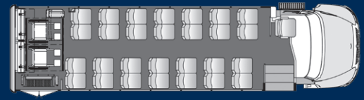
28 Passenger 2 Wheelchair 2 Passenger Foldaway and 4 Passenger Flip Seats Plus Driver
