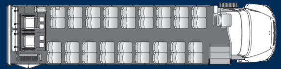
36 Passenger 2 Wheelchair 2 Passenger Foldaway and 4 Passenger Flip Seats Plus Driver
